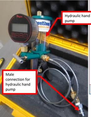
A typical hydraulic system should include an isolation or "shut-off" valve, a connection for a hydraulic hand pump or portable hydraulic power unit, the chart recorder's electronic transducer, and your calibrated Master Gauge.
