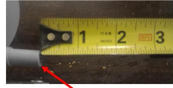
Measure cable length from transducer base to the end of cable.
